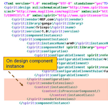
Figure 5: Context labels in a IP-XACT design file
