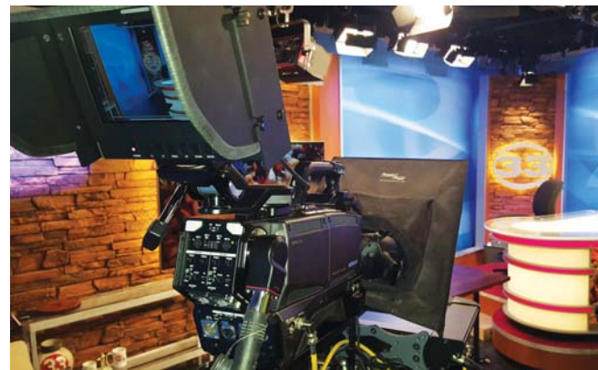
Photo 2: CMOS imaging technology has been implemented in its Z-HD5500 and SK-HD1800 HDTV camera models.
