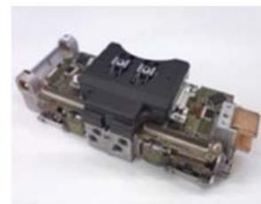
Optical head system DCHS (Dual Channel Head System)
